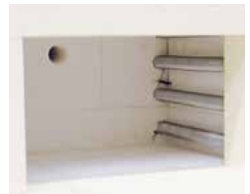
Furnace lining with high-quality lightweight refractory brick insulation
